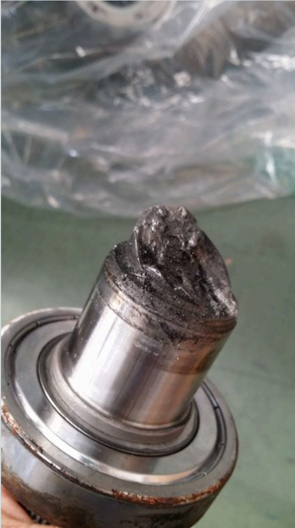
Figure 1 – Fracture surface of the drive shaft between operating mechanism and breaker body. Site photograph.
